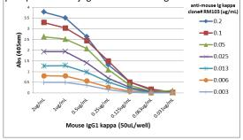
A titer ELISA of mouse  $lgG1\kappa$ . The plate was coated with different amounts of mouse  $lgG1\kappa$ . A serial dilution of RM103 was used as the primary antibody. An alkaline phosphatase conjugated anti-rabbit lgG as the secondary antibody.
